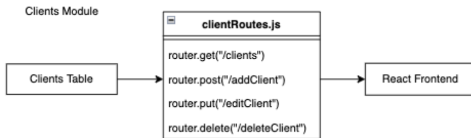
Figure 4.2: Diagram showing the UML interactions for this module
